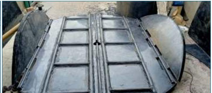
**HDPE SHEET VESSEL COVER FOR HINGE TYPE**
